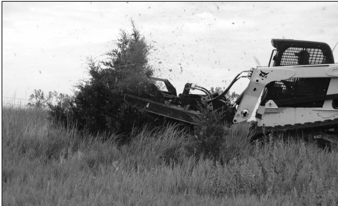
Using a new mechanical method, Scott McDowell of Loup Valley Construction, Inc., mulches a red cedar. The quick process will give landowners another option in controlling the invasive tree. (Kendra Veirs photo)
